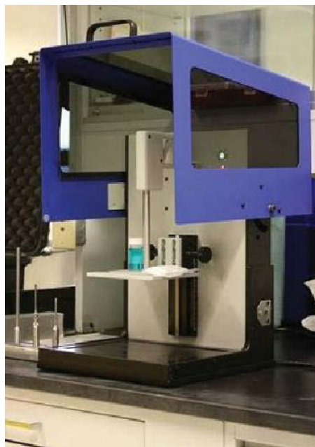
Figure 1 – The TouchRaman MOMO has an open design to enable collaboration of several students using Raman spectroscopy. This design is also compatible with bringing large samples to the height-adjustable assay stage. The outer cover protects users from stray laser light.
