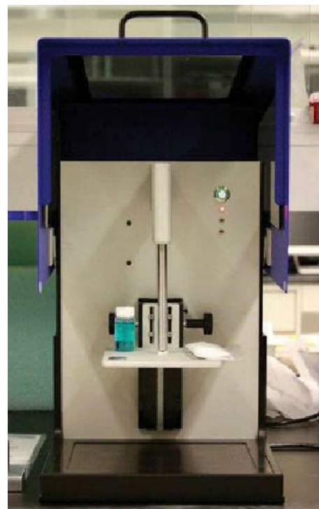
Figure 2 – Close-up of the height-adjustable BallProbe sample stage. The lower end of the vertical probe end is terminated with a high-purity sapphire ball lens. Laser light is transmitted to the ball by a metal encased light pipe (center). Light passes through the patented spherical lens and into the sample region immediately below the sapphire ball. In this case, a solid pill is located immediately under the BallProbe; the probe is equally effective with liquids, slurries and powders. When a sample is excited using a laser, Stokes (Raman) scattering occurs. Part of the Stokes scattered light reenters the sapphire ball and up the optics to the detector where the intensity is recorded as a function of wavelength, yielding a Raman spectrum.
